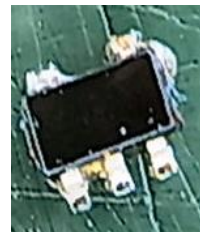
excessive solder residues resulting in bridging neighboring pins / leads 2)
