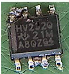
severe package defects & cut-off pins / leads 2)
