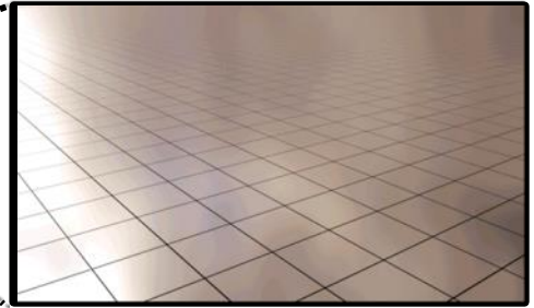
Array of mirrors (5.4 \mu m TRP)
