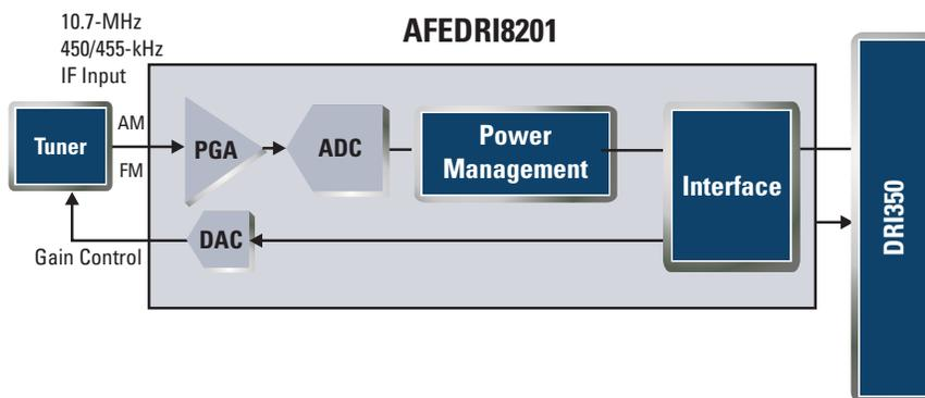
*ADC and DAC integrated to provide precision AM/FM and HD Radio digitization.*
