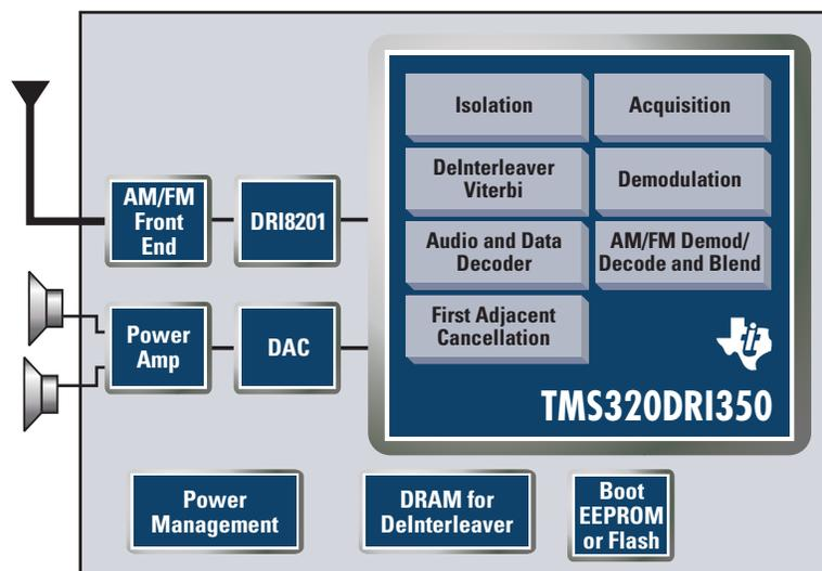
The TMS320DRI350 baseband integrates the baseband processing for both HD Radio and AM/FM on a single device. The DRI8201 samples and downconverts the intermediate frequency (IF) from the AM/FM front end.
