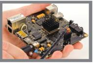
Connect the supplied power cable to the processor board as shown (for simplicity only the processor board is shown). Connect the 12-volt power supply cable to an AC power source.
