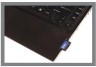
To prepare your workstation for software development, power off the kit, remove the microSD card and insert it into your Ubuntu Linux workstation (adapter maybe required). If your workstation does not include an SD slot, USB SD card adapters are readily available. Follow the instructions to the right
