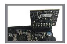
Optional: Connect the camera module to the camera header of the IDK, with the camera sensor facing away from the IDK.
