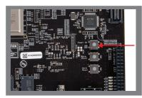
Push the power on push button (SW3) to run the IDK.
