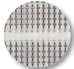
A general-purpose area which can be used as a proto-board
