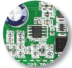
A wide-input non-synchronous buck-type DC/DC controller
