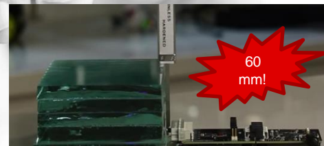
Sense through 60mm thick glass
