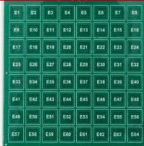
Tiny sensors (3x5mm 2 )
