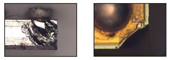
Examples of severe mechanical damage to WCSP device
