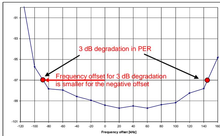
**Figure 2. Definition of Frequency Offset which gives 3 dB Degradation in PER (unsymmetrical frequency offset)**
