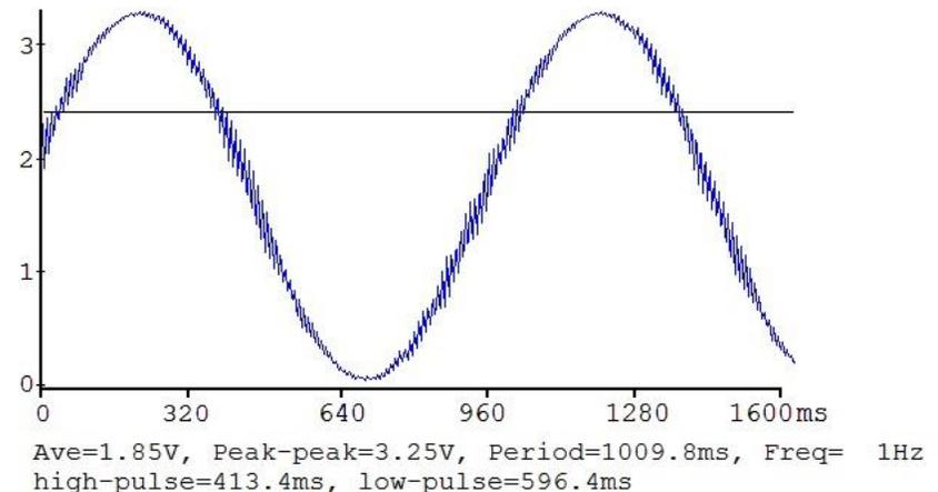
Figure 6. Example analog output of the PWM DAC.
