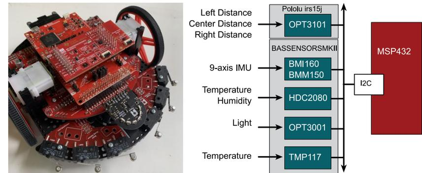
Figure 1. RSLK with the Pololu OPT3101 Time of Flight module used to measure distance, and the TI BP-BASSENSORSMKII Boosterpack used to measure acceleration, rotation, magnetic field, temperature, humidity, and light intensity.
