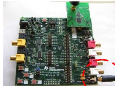
Connect an amplifier to line out or connect a headphone to the mini jack of the AudioEB with the CC85xxEM or the CC85xx-CC2590 with the "SLAVE" label plugged in.
