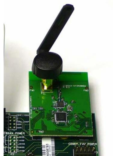
Connect the CC85xxEM or the CC85xx-CC2590EM marked MASTER (label attached on the backside of the board). These boards are pre-programmed with master firmware. Attach the antenna to the SMA connector.
