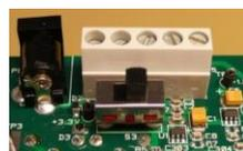
If EB and EM are powered from different sources as described in 4a-4c, the switch should be set to the rightmost position.
