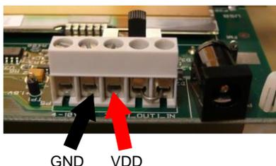
Connect a 3.3 V voltage source between the 3.3 V and 0 V terminals. 3.3 V is the middle terminal.
