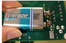
Alternatively, connect a 9 Volt, non-rechargeable, alkaline battery to the battery connector on the bottom side of the board.
