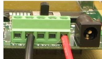
As noted in 4a, remove the strap on P5 and connect the external power supply as shown in the picture above. The red wire is the positive supply and the black wire is GND.
