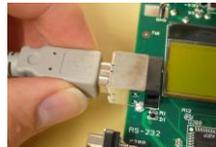
Connect the EB to a USB port on a PC.
