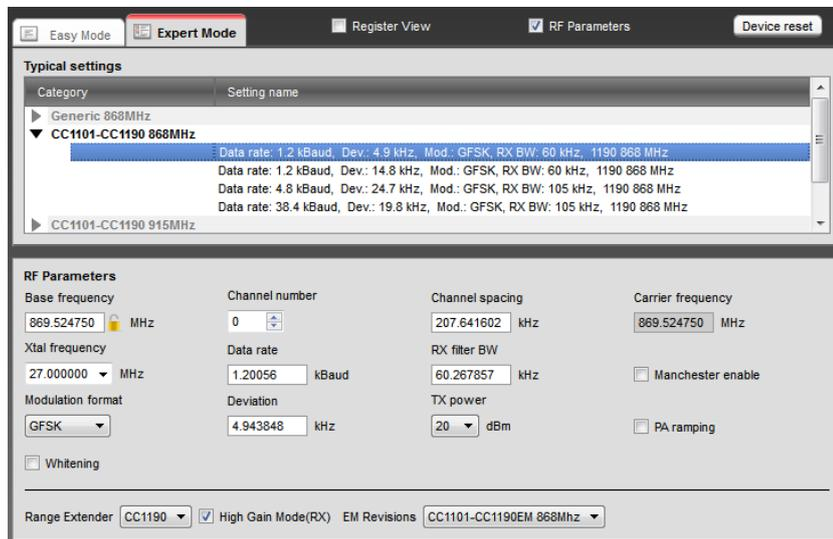
In order to control the CC1190 select CC1190 as “Range Extender” and select the appropriate “EM Revisions” as shown (either 869 or 915 MHz). You can now use all the features in Studio as for a standalone EM. Test the performance of the radio using some of these features:
