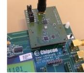
Insert the EM into the EB. Attach the antenna firmly.
