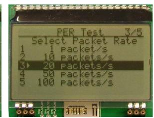
On the transmitter, select the desired packet rate
