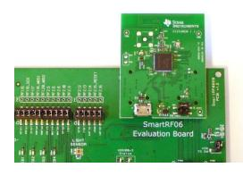
Insert a CC2538EM board into the SmartRF06EB as shown above. **NB! Note the jumper on the upper row on the header on the CC2538EM.**
