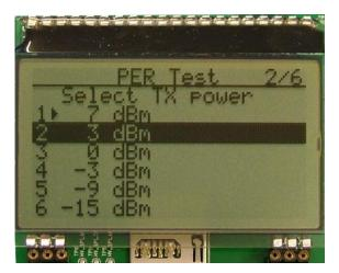
On the transmitter, select desired output power.
