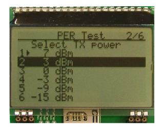
On the transmitter, select desired output power.
