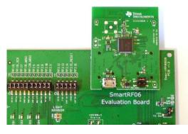
Insert a CC2538EM board into the SmartRF06EB as shown above. **NB! Note the jumper on the upper row on the header on the CC2538EM.**
