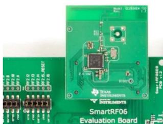
Insert a CC2650EM board into the SmartRF06EB as shown above.
