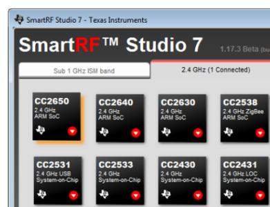
After installing the tool, connect the EB to the PC using the USB cable and start SmartRF Studio. Select the "2.4 GHz" tab and click the refresh ("Find device") button in the lower right corner. Studio will now find the connected SmartRF06EB. Double click on the detected SmartRF06EB to launch the CC2650 device control panel.
