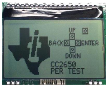
Turn on power with the Main Power switch. You should now see the Texas Instruments logo and a short description of the buttons on the LCD. Pushing any of the five buttons on the board will take you to the main menu.
