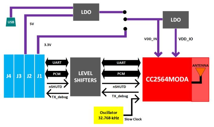
Figure 3. BOOST-CC2564MODA Block Diagram
