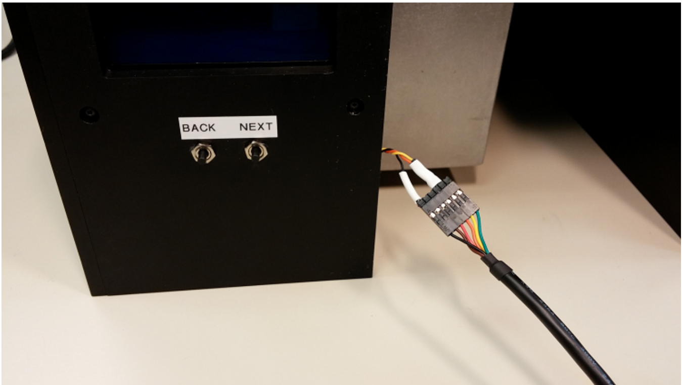
Figure 3-10. TTL-232R-3V3 Connected To DLP 3D Printer
