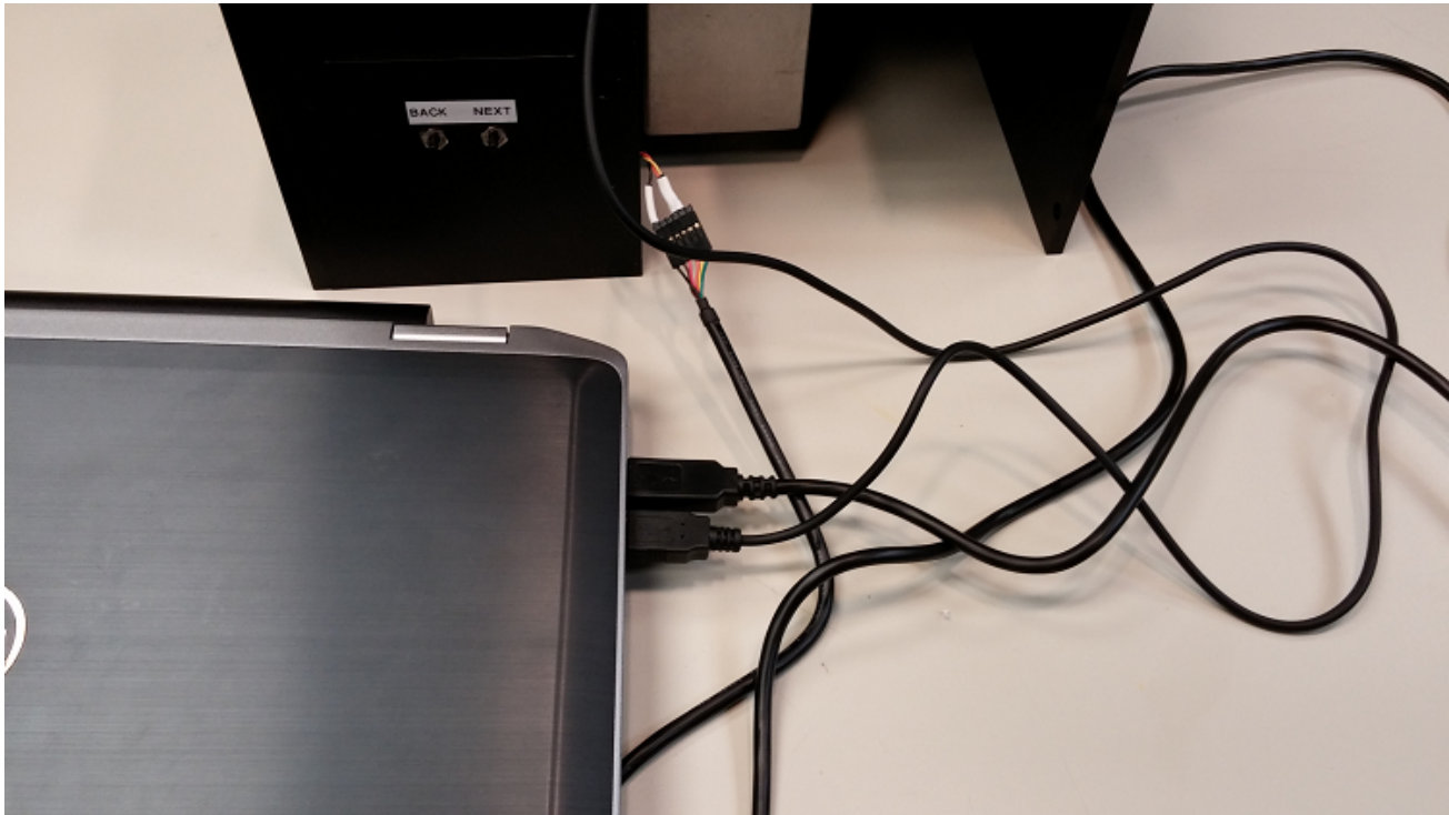
Figure 3-12. LightCrafter 4500 And TTL-232R-3V3 Cable Connected To PC
