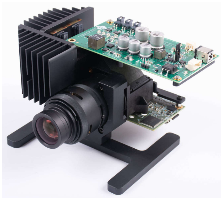
Figure 3-1. DLP5530PROJTGQ1EVM Optical Module
