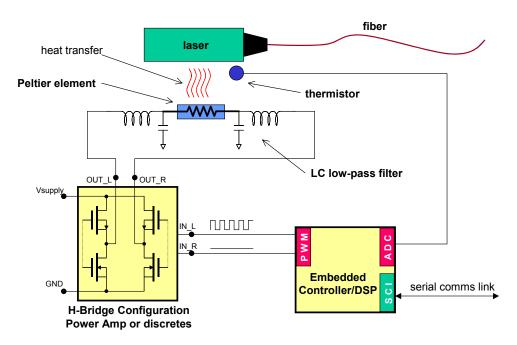
Figure 4. Thermoelectric Cooler Block Diagram.
