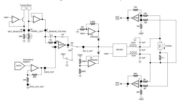
Figure 6. TEC Control Loop.
