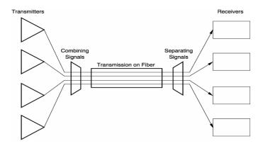
Figure 1. DWDM Multiplexes Many Signals Onto One Fiber.
