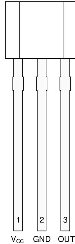
**Figure 4-2. LPG Package 3-Pin TO-92 Top View**
