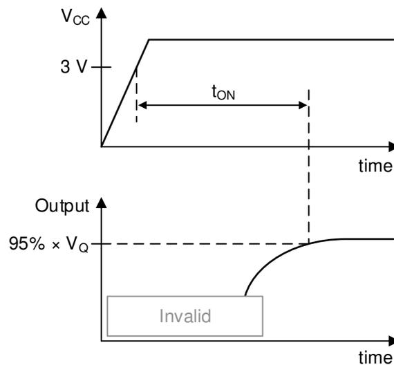
Figure 6-4.  $t_{ON}$  Definition
