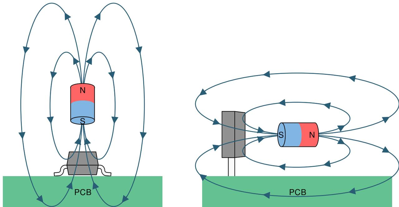
**Figure 6-2. The Flux Direction for Positive B**
