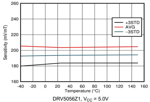
**Figure 5-18. Sensitivity vs Temperature**
