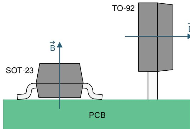
**Figure 6-1. Direction of Sensitivity**
