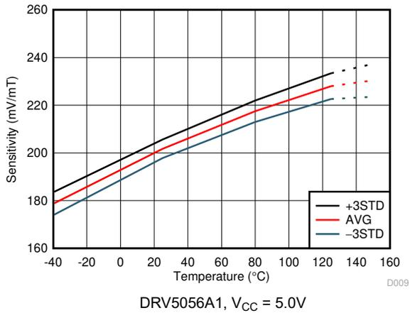
Figure 5-7. Sensitivity vs Temperature
