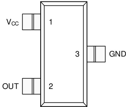
**Figure 4-1. DBZ Package 3-Pin SOT-23 Top View**
