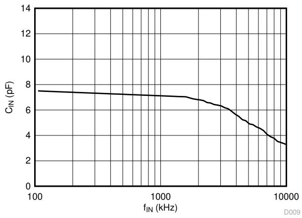
Figure 6-8. Input Capacitance vs Input Signal Frequency
