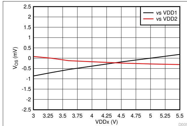
Figure 6-5. Input Offset Voltage vs Supply Voltage
