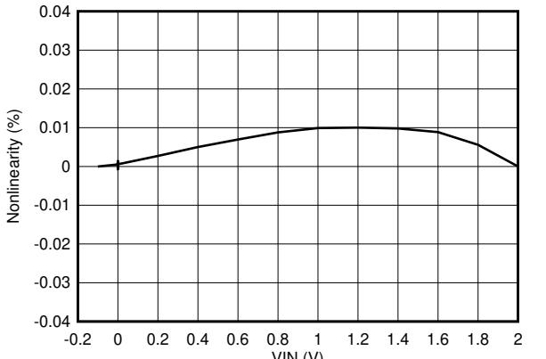
Figure 6-16. Nonlinearity vs Input Voltage
