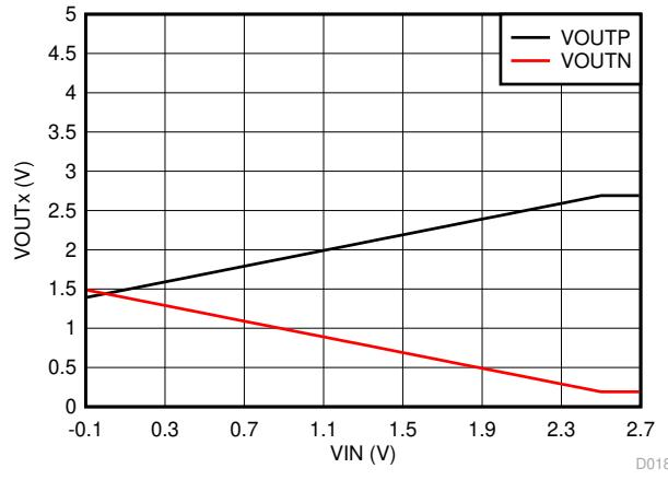
Figure 6-15. Output Voltage vs Input Voltage
