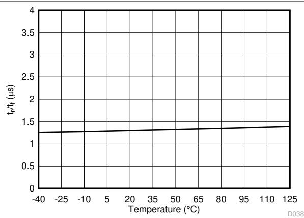
Figure 6-33. Output Rise and Fall Time vs Temperature
