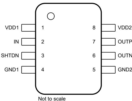
**Figure 5-1. DWV Package, 8-Pin SOIC (Top View)**
