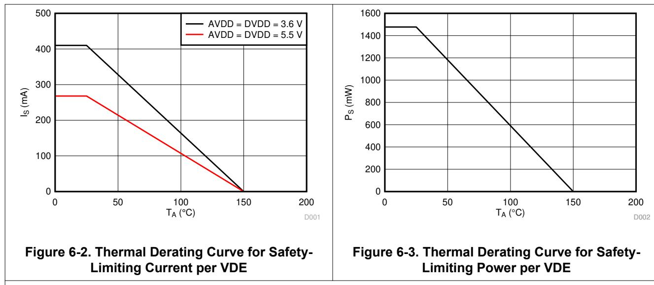
**Figure 6-2. Thermal Derating Curve for Safety-Limiting Current per VDE**
