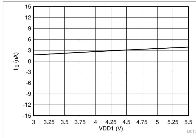
Figure 6-9. Input Bias Current vs High-Side Supply Voltage
