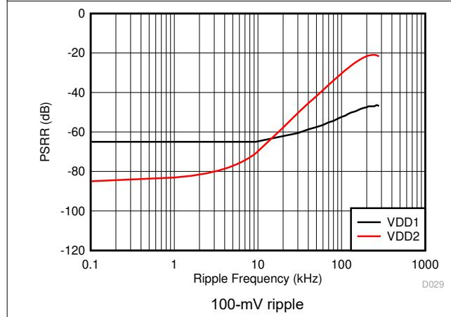
Figure 6-25. Power-Supply Rejection Ratio vs Ripple Frequency
