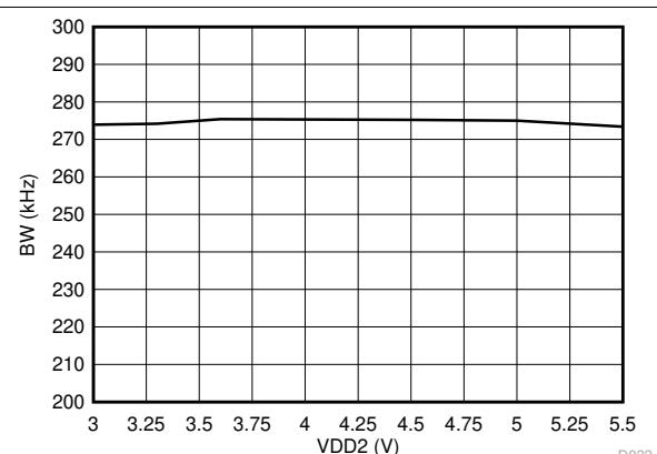
Figure 6-28. Output Bandwidth vs Low-Side Supply Voltage
