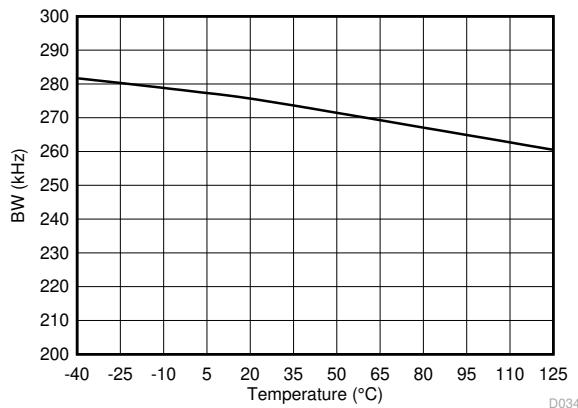
Figure 6-29. Output Bandwidth vs Temperature
