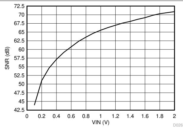
Figure 6-22. Signal-to-Noise Ratio vs Input Voltage
