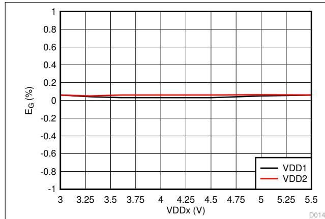
Figure 6-11. Gain Error vs Supply Voltage
