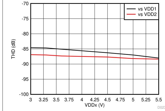
Figure 6-19. Total Harmonic Distortion vs Supply Voltage
