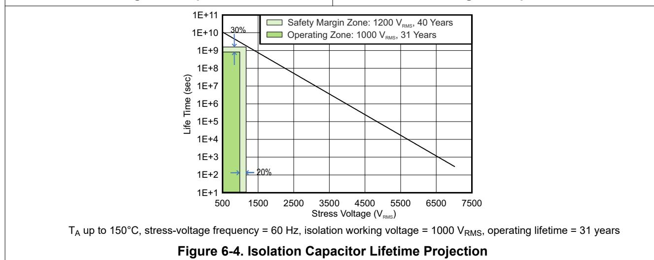
**Figure 6-4. Isolation Capacitor Lifetime Projection**
