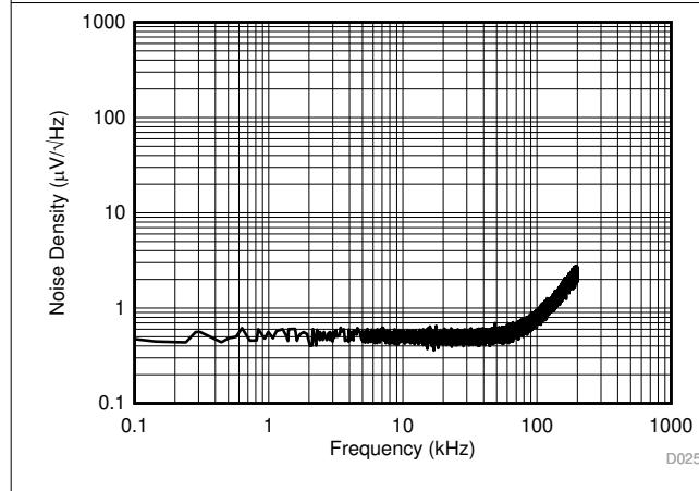
Figure 6-21. Input-Referred Noise Density vs Frequency
