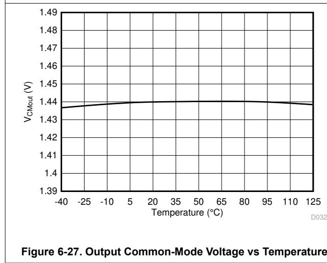
Figure 6-27. Output Common-Mode Voltage vs Temperature
