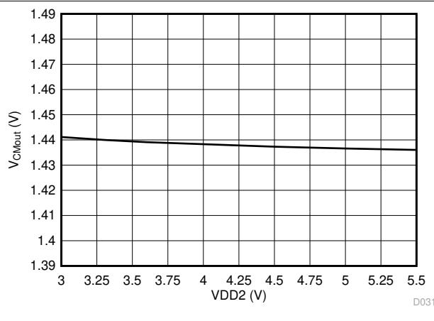
Figure 6-26. Output Common-Mode Voltage vs Low-Side Supply Voltage
