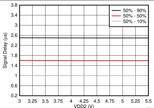
Figure 6-34. IN to OUTP, OUTN Signal Delay vs Low-Side Supply Voltage
