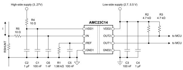
Figure 8-9. Decoupling of the AMC23C14
