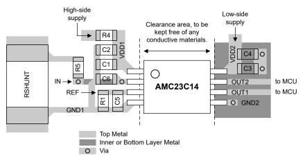
Figure 8-10. Recommended Layout of the AMC23C14
