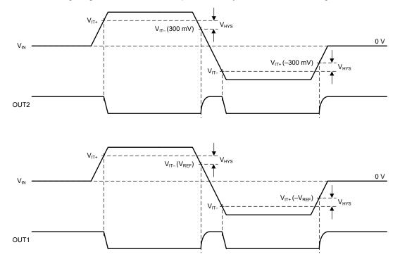
Figure 7-1. Switching Thresholds and Hysteresis
