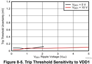
Ripple Voltage (Cmp0, f<sub>RIPPLE</sub> = 10 kHz)
