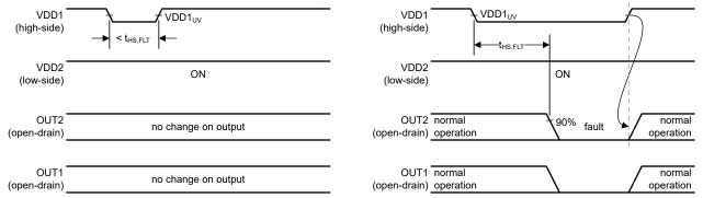
Figure 7-11. Output Response to a Short Brownout Figure 7-12. Output Response to a Long Brownout Event on VDD1
