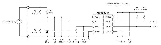
Figure 8-2. Using the AMC23C14 for Overvoltage and Undervoltage Detection
