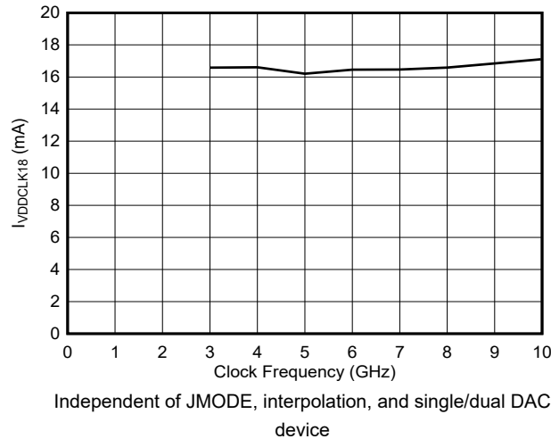
Figure 6-217. VDDCLK18 Current vs Clock Frequency
