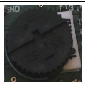
Figure 4-5. Potentiometer Position for Creating 14.3kΩ ADJ Resistance
