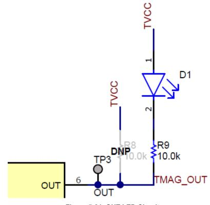
Figure 5-21. OUT LED Circuit
