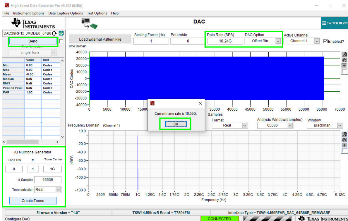
Figure 3-9. HSDCpro Generating the Tone and Sending it to the DAC.
