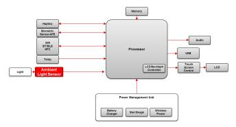
Figure 1. Smart Watch Display Block Diagram
