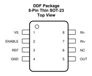
Figure 4-2. Pin Diagram (DDF-8 Package)
