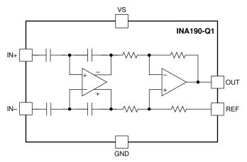
Figure 1-1. Functional Block Diagram
