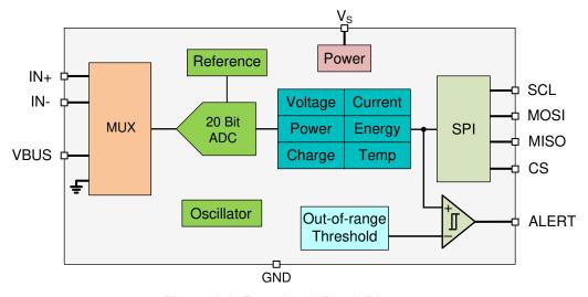
Figure 1-1. Functional Block Diagram
