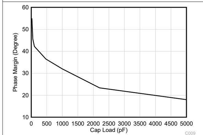
Figure 5-29. Phase Margin vs Capacitive Load
