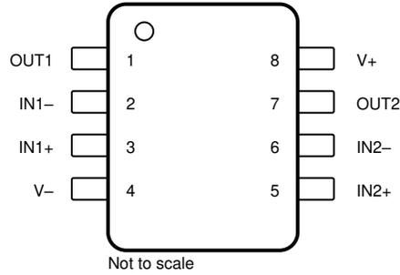
**Figure 4-3. TLV9352-Q1 D, PW and DGK Package,
