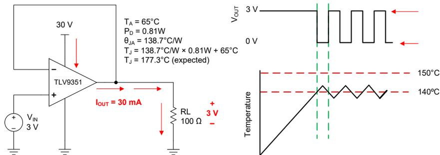
**Figure 6-4. Thermal Protection**
