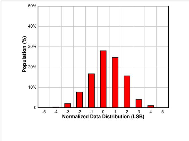
**Figure 7-15. Data Distribution With 3-ms Conversion Time and Averaging Off in 16-Bit Format**
