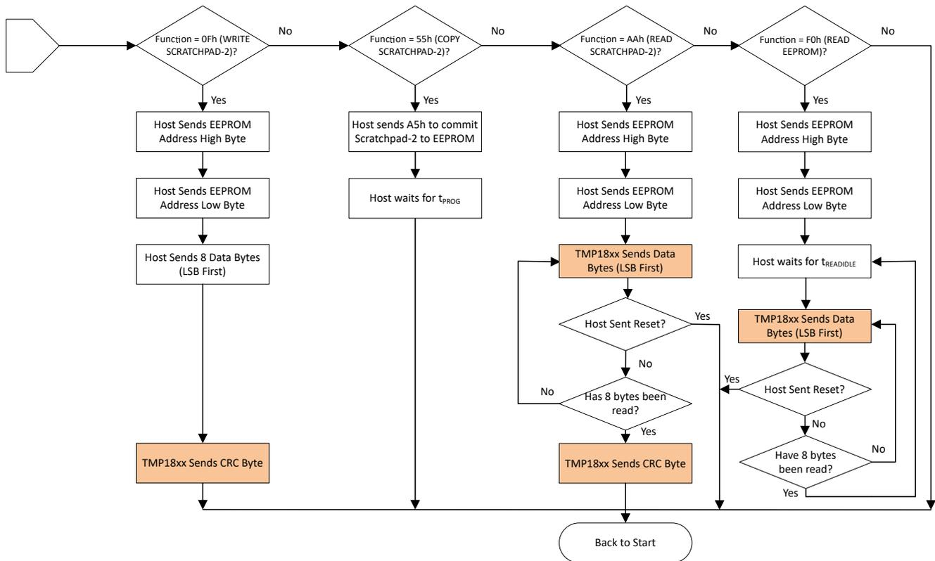
Figure 8-23. Function Phase Flowchart for Memory Access
