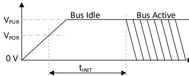
**Figure 7-5. Bus Powered Initialization Timing Diagram**
