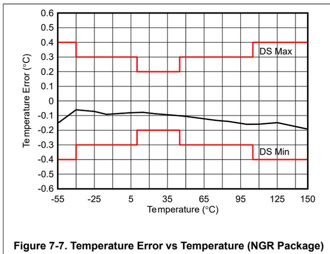
Figure 7-7. Temperature Error vs Temperature (NGR Package)
