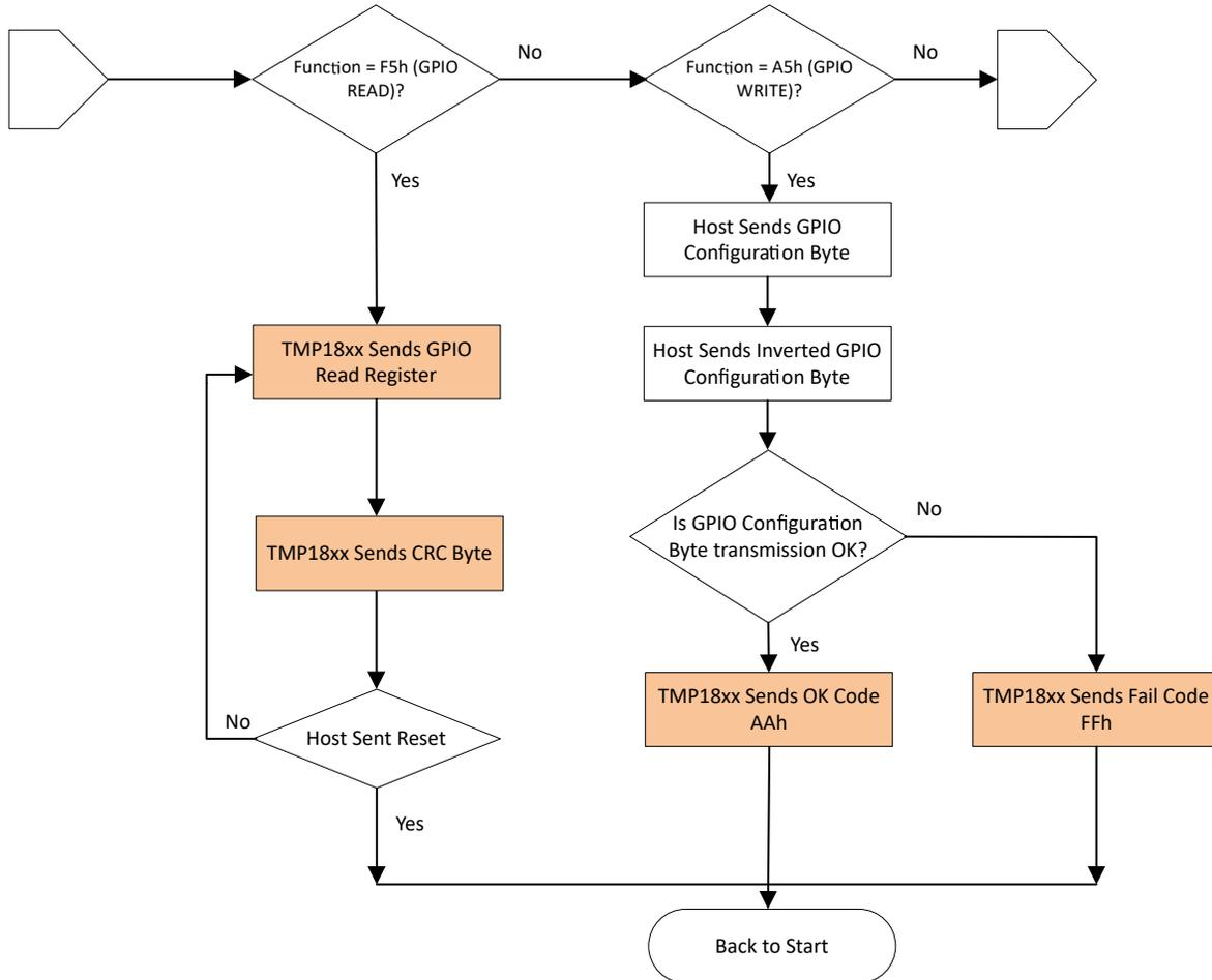
Figure 8-24. Function Phase Flowchart for IO Access
