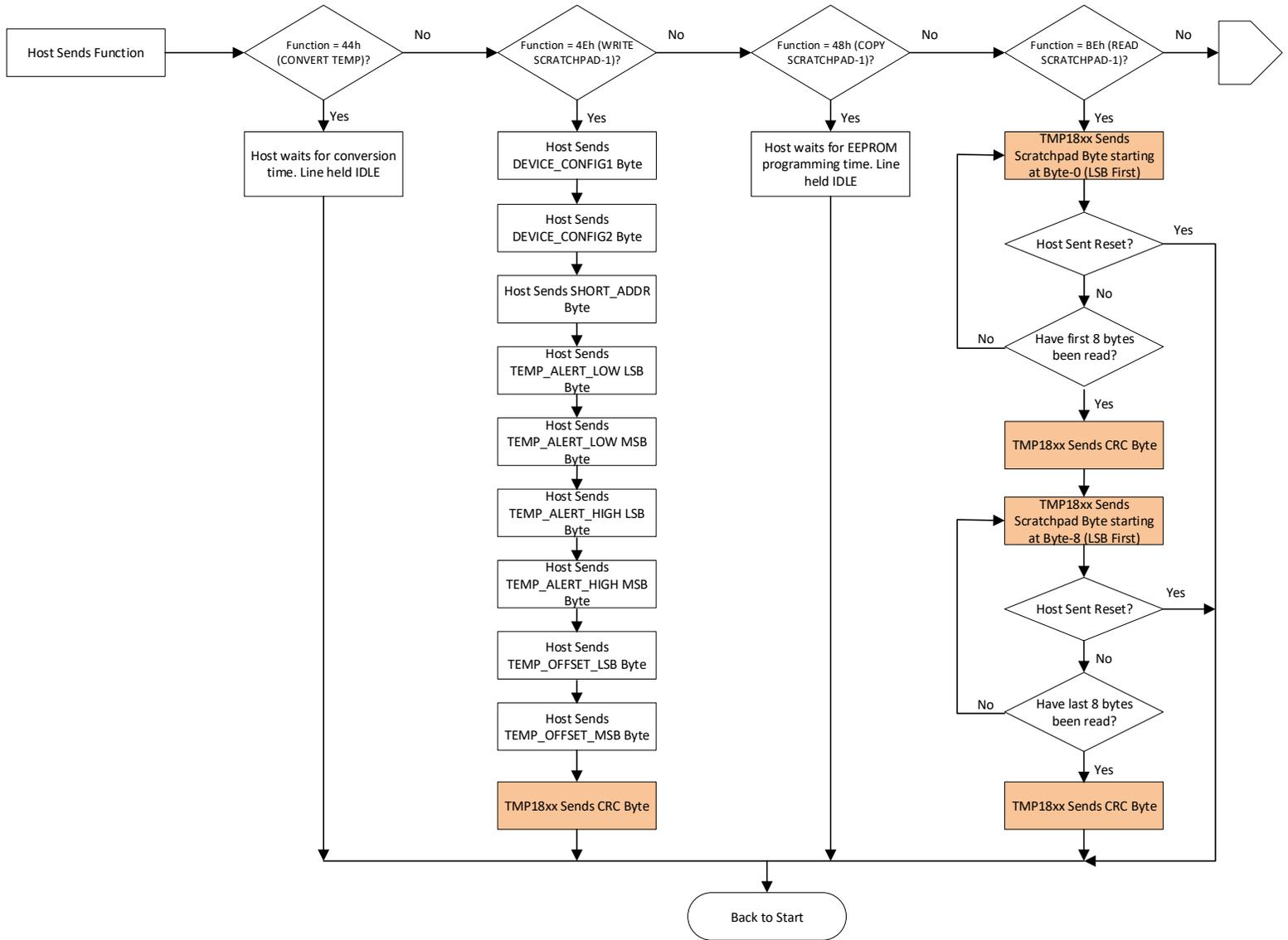
Figure 8-22. Function Phase Flowchart for Register Space
