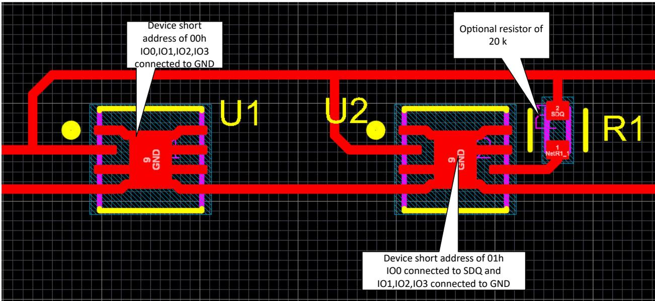
Figure 9-6. IO Hardware Address in Bus Powered Mode
