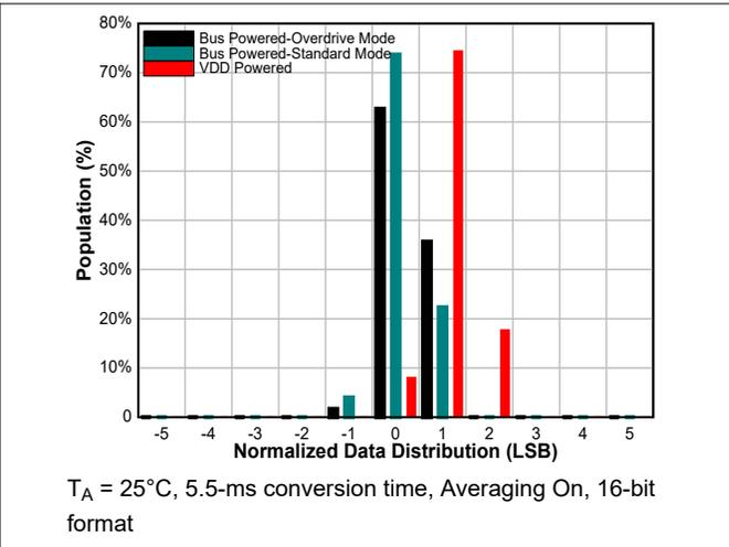
**Figure 7-16. Data Distribution for Power Mode and Bus Speed**
