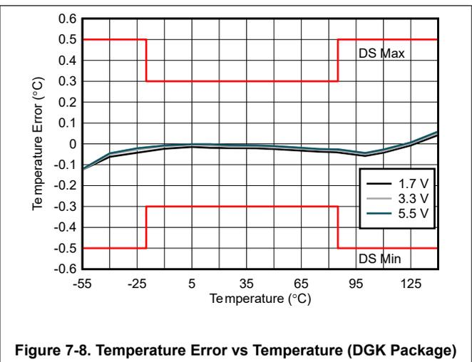
Figure 7-8. Temperature Error vs Temperature (DGK Package)
