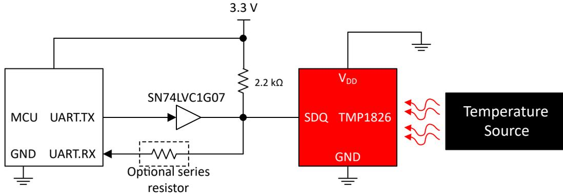
Figure 9-3. Using UART to Interface TMP1826
