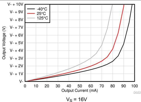
**Figure 5-17. Output Voltage Swing vs Output Current (Sinking)**
