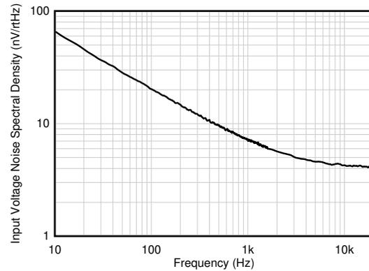
Figure 5-26. Input Voltage Noise Spectral Density vs Frequency
