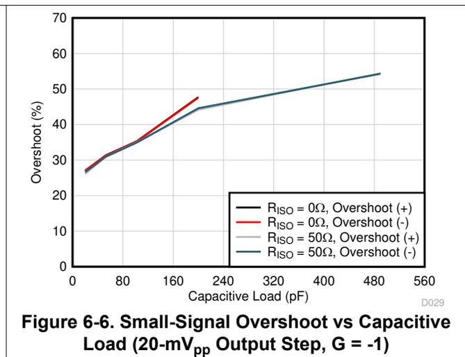
Figure 6-6. Small-Signal Overshoot vs Capacitive Load (20-mV<sub>pp</sub> Output Step, G = -1)
