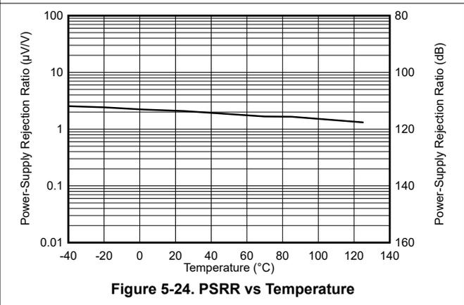
**Figure 5-24. PSRR vs Temperature**
