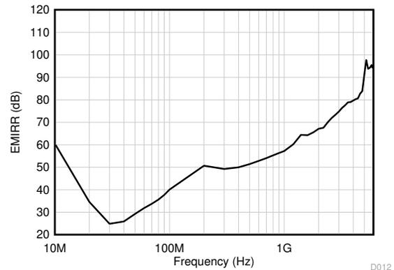
**Figure 5-40. EMIRR (Electromagnetic Interference Rejection Ratio) vs Frequency**
