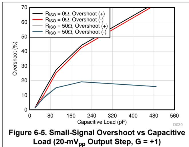
Figure 6-5. Small-Signal Overshoot vs Capacitive Load (20-mV<sub>pp</sub> Output Step, G = +1)
