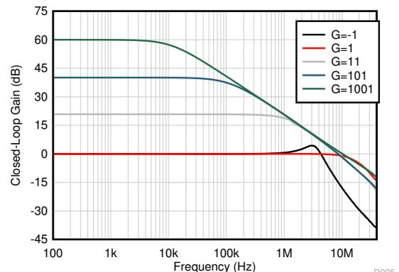
**Figure 5-12. Closed-Loop Gain vs Frequency**
