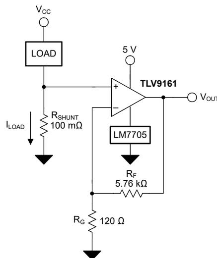
Figure 7-1. TLV9161 in a Low-Side, Current-Sensing Application
