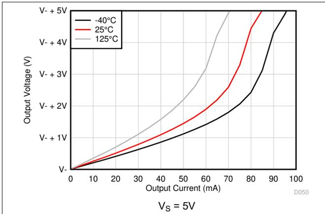
**Figure 5-19. Output Voltage Swing vs Output Current (Sinking)**
