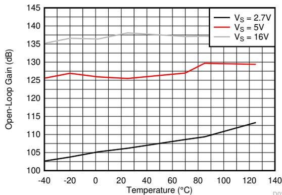
Figure 5-29. Open-Loop Voltage Gain vs Temperature (dB)
