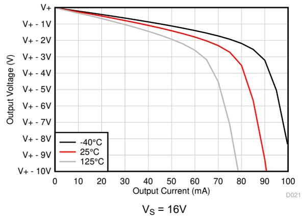
**Figure 5-16. Output Voltage Swing vs Output Current (Sourcing)**
