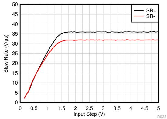
**Figure 5-15. Slew Rate vs Input Step Voltage**
