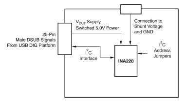
Figure 2-2. INA220\_Test\_Board Block Diagram
