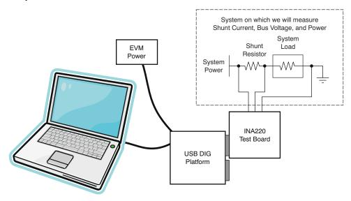
Figure 2-1. INA220EVM Hardware Setup
