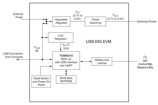
Figure 2-4. USB\_DIG\_Platform Theory of Operation
