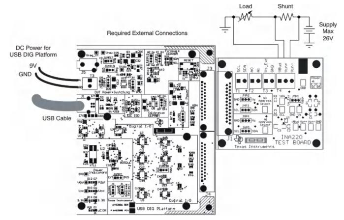
Figure 3-1. Typical Hardware Connections
