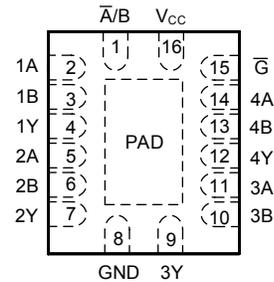
Figure 4-2. WBQB Package, 16-Pin WQFN (Transparent Top View)
