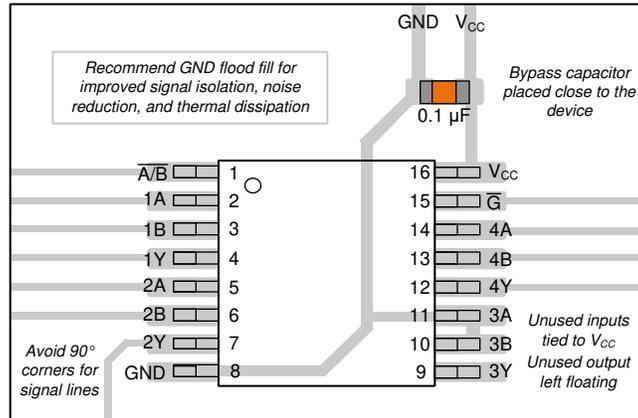
Figure 8-3. Example Layout for the SN74AHCT157-Q1
