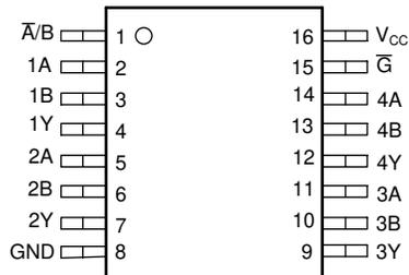
Figure 4-1. PW Package, 16-Pin TSSOP (Top View)
