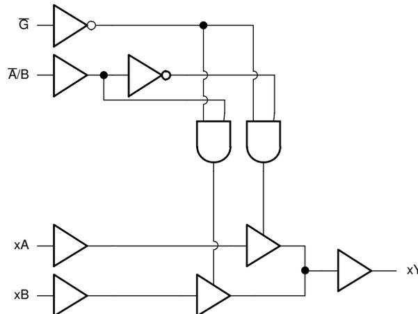
Figure 7-1. Logic Diagram (Positive Logic) for SN74AHCT157-Q1
