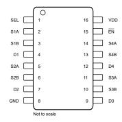
Figure 3. Pin Diagram (SOT-23 Package)
