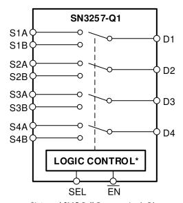
\*Internal 6M $\Omega$  Pull-Down on Logic Pins
