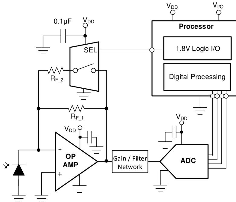
Figure 9-4. Configurable Gain Setting of a TIA Circuit
