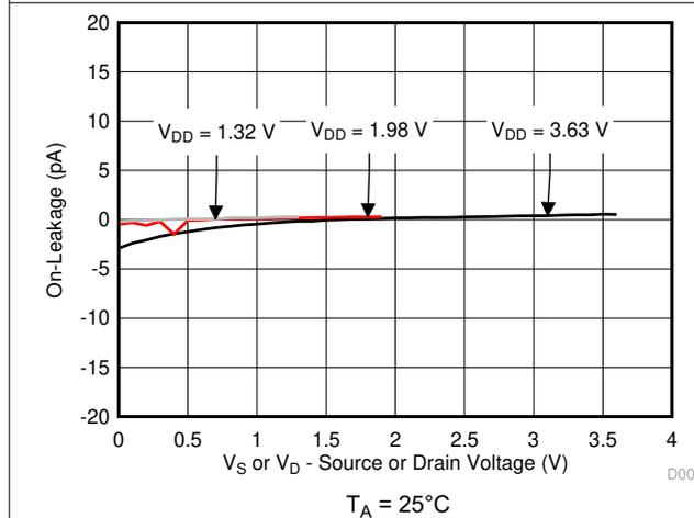
Figure 6-5. On-Leakage vs Source or Drain Voltage
