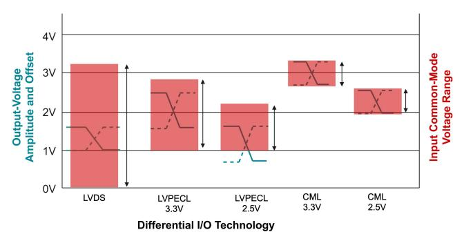
Figure 2. Differential Signaling Standard Inputs Supported by DS90LVRA2 LVDS, CML, LVPECL
