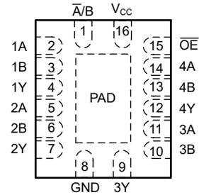
Figure 5-2. BQB Package, 16-Pin WQFN (Transparent Top View)
