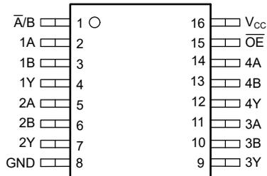
Figure 5-1. PW Package, 16-Pin TSSOP (Top View)
