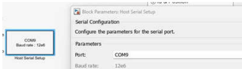
Figure 2-6. Update the COM Port Number for the Host Model
