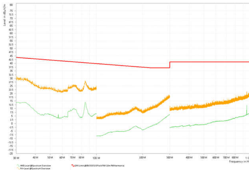
Figure 2-22. Radiated Emissions – Standby, VM = 12V, INx = 5V, No Load
