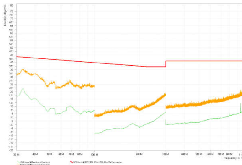
Figure 2-24. Radiated Emissions – Active With PWM, VM = 12V, INx = 3.3V At 20kHz, 48Ω Load
