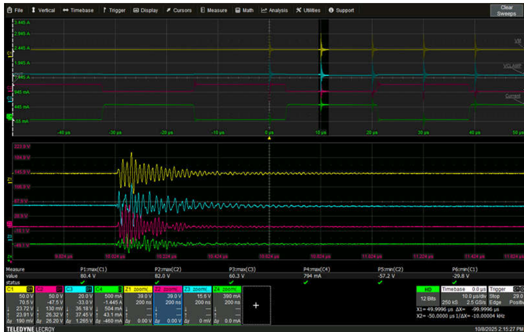
Figure 2-11. Captured Surge Waveform With Driver In OFF State 1500V Zoomed In
