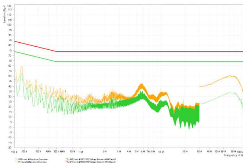
Figure 2-19. Conducted Emissions – Active With PWM, VM = 12V, INx = 3.3V At 20kHz, 48Ω Load
