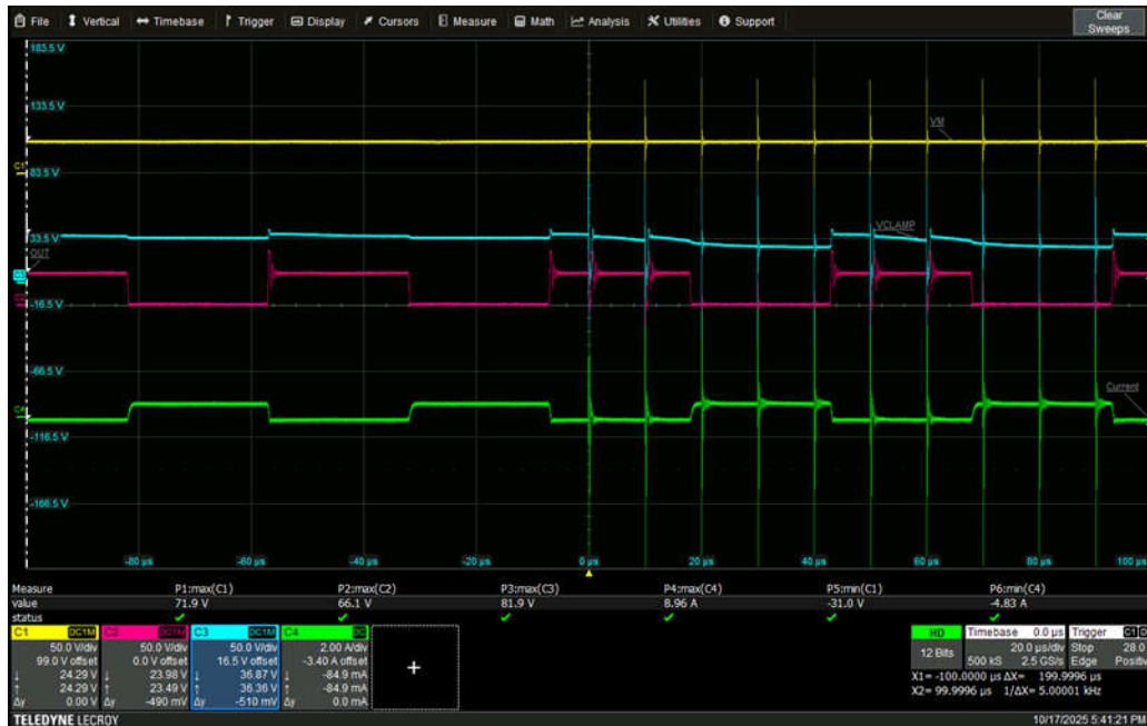
Figure 2-13. EFT at 2.5kV on OUT Line
