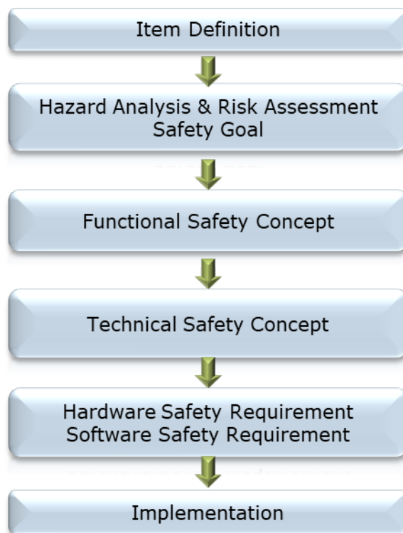
Figure 1-2. Safety Requirement Development Process
