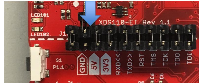
Figure 6. MSP432 LaunchPad with +5V jumper removed.
