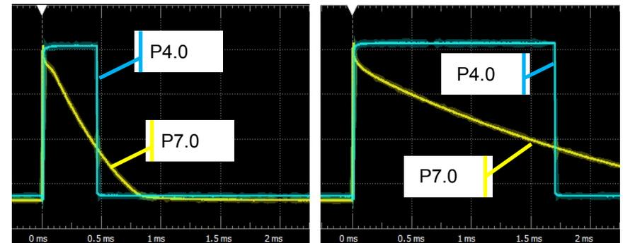
Figure 11 Left side measured with white surface, right side measurements with black surface. If you read P7.0 at 1ms, it will be low for white and high for black.
