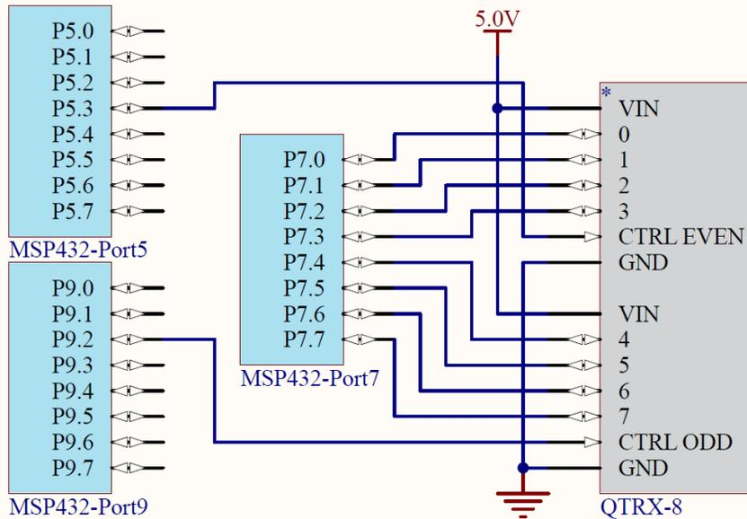
Figure 8 The 8-channel line sensor is interfaced to Ports 5, 7, and 9. These connections are made on the TI-RSLK chassis board. Sensor 0 (P7.0) is on the right, and sensor 7 (P7.7) is on the left.
