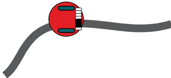
Figure 3. Robot with eight line sensors and two wheel motors.
