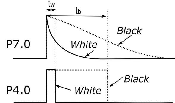
Figure 10. Conversion of light to voltage, and voltage to binary.
