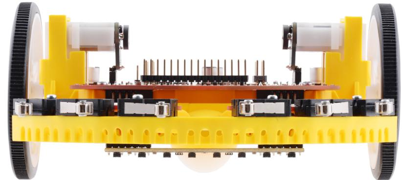
Figure 1. QTRX mounted on bottom of robot, 3mm above the floor. Notice, the sensor does not extend over the battery compartment.
