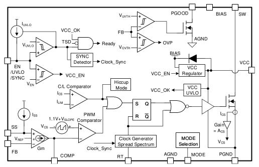
Figure 1-1. Functional Block Diagram
