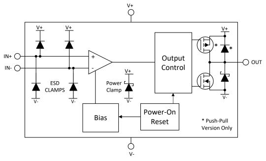
Figure 1-1. Functional Block Diagram
