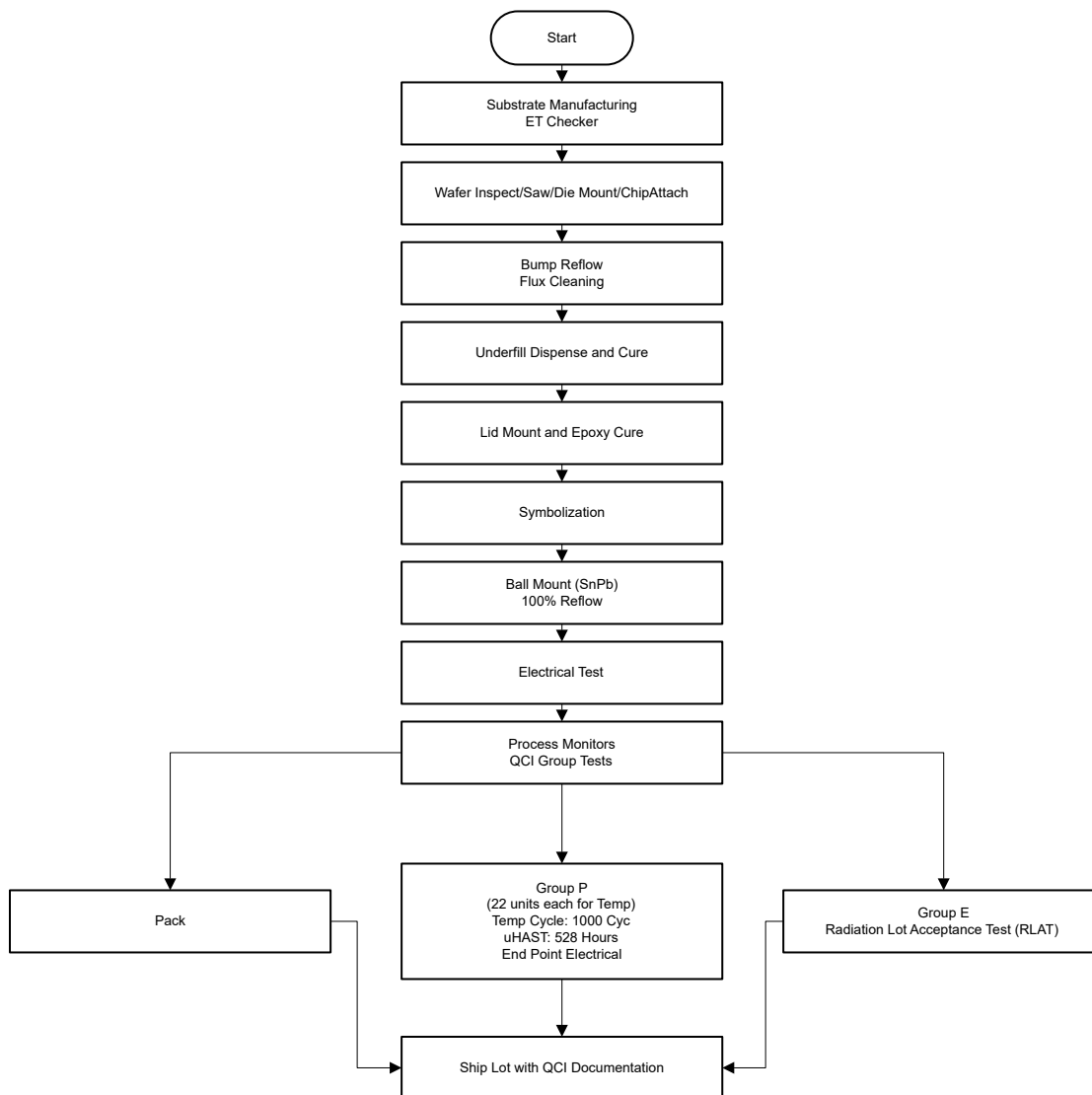
Figure 1-1. AFE7950-SEP Space Enhanced Plastic Production Flow Chart
