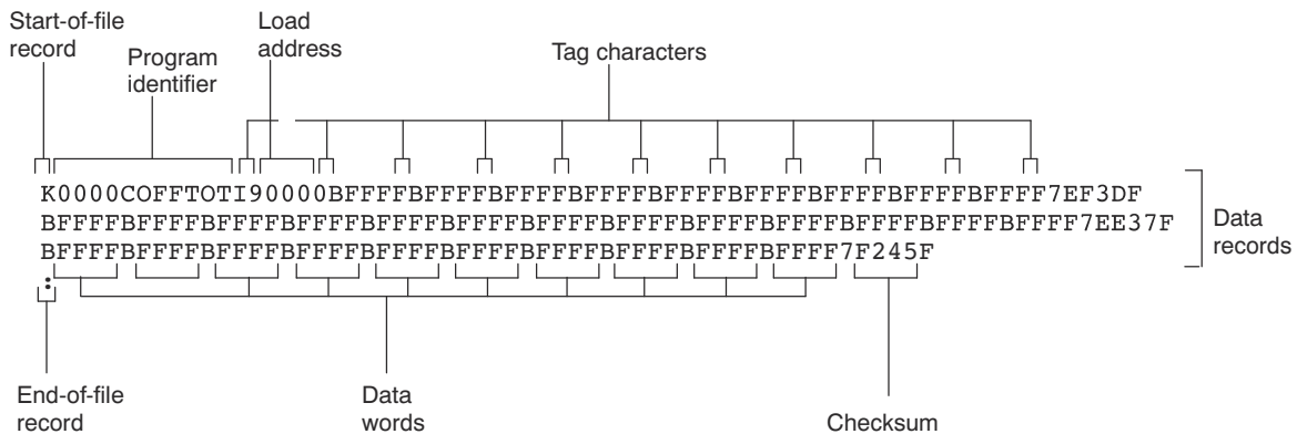
Figure 12-10. TI-Tagged Object Format
