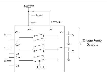
Figure 3. Charge Pump Regulator
