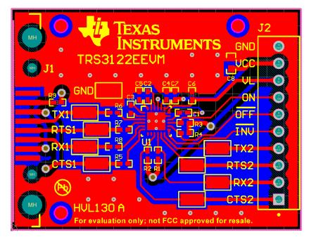
Figure 4. TRS3122E 2-Layer Metal Example Layout
