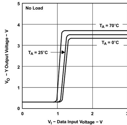
Figure 5-10. Y Output Voltage vs Data Input Voltage
