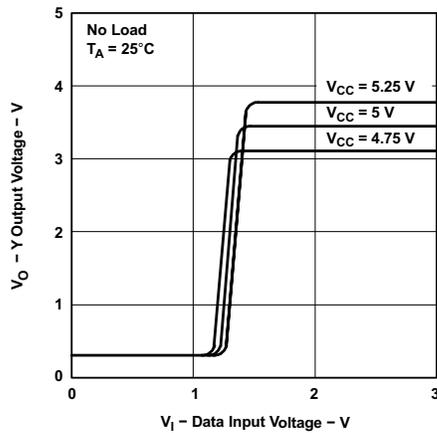
Figure 5-9. Y Output Voltage vs Data Input Voltage
