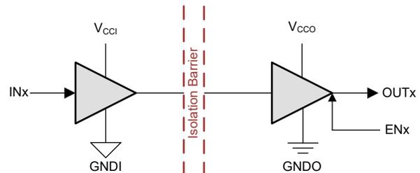
V<sub>CCI</sub>=Input supply, V<sub>CCO</sub>=Output supply
