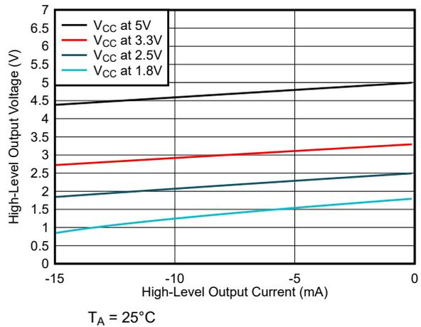
Figure 6-9. High-Level Output Voltage vs High-level Output Current
