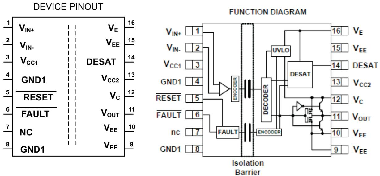
Figure 1. ISO5500 Pinout and Functional Block Diagram
